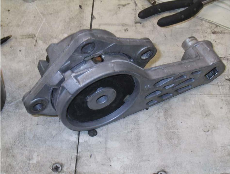
3. Trim about 1 inch off of the "maximum travel" stops on the bottom of both the tensioners (pic below).
