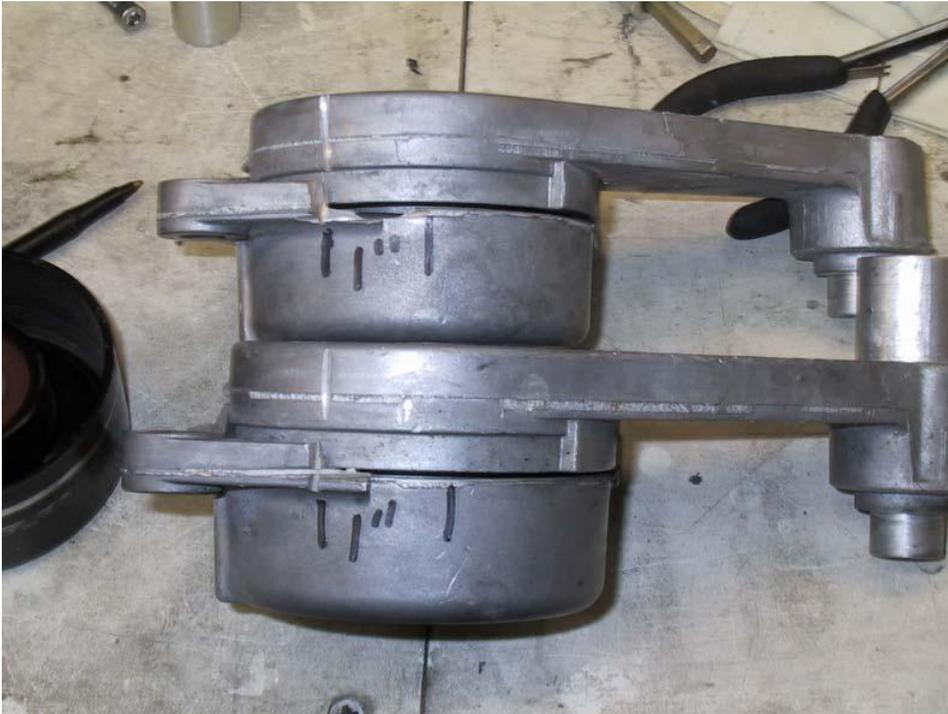
4. Drill the pulley bolt hole all the way through on the INSIDE tensioner. DO NOT DRILL THE HOLE/TREADS OUT OF THE OUTSIDE TENSIONER!!!!
